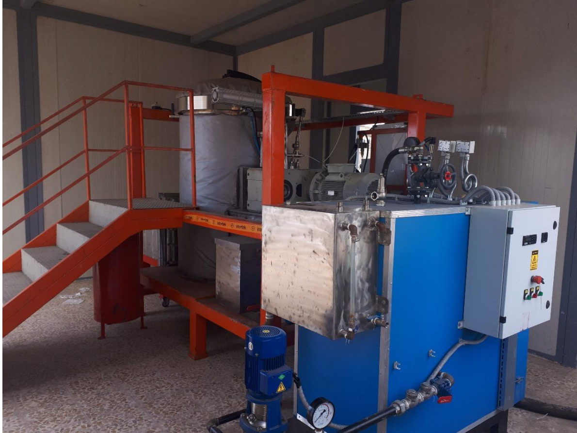
Picture.4. ARI-550:250 liters/cycle manufactured for UNDP Iraq Al-Qayara Hospital
